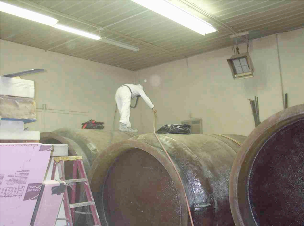
An air hose is used to clean the perlite dust off of the cryostats. The 16½" diameter fiberglass plate for the filter hole is drilled in the center and 11" copper pipe with hand ball valve (from Home Depot) is fitted to the opening.
