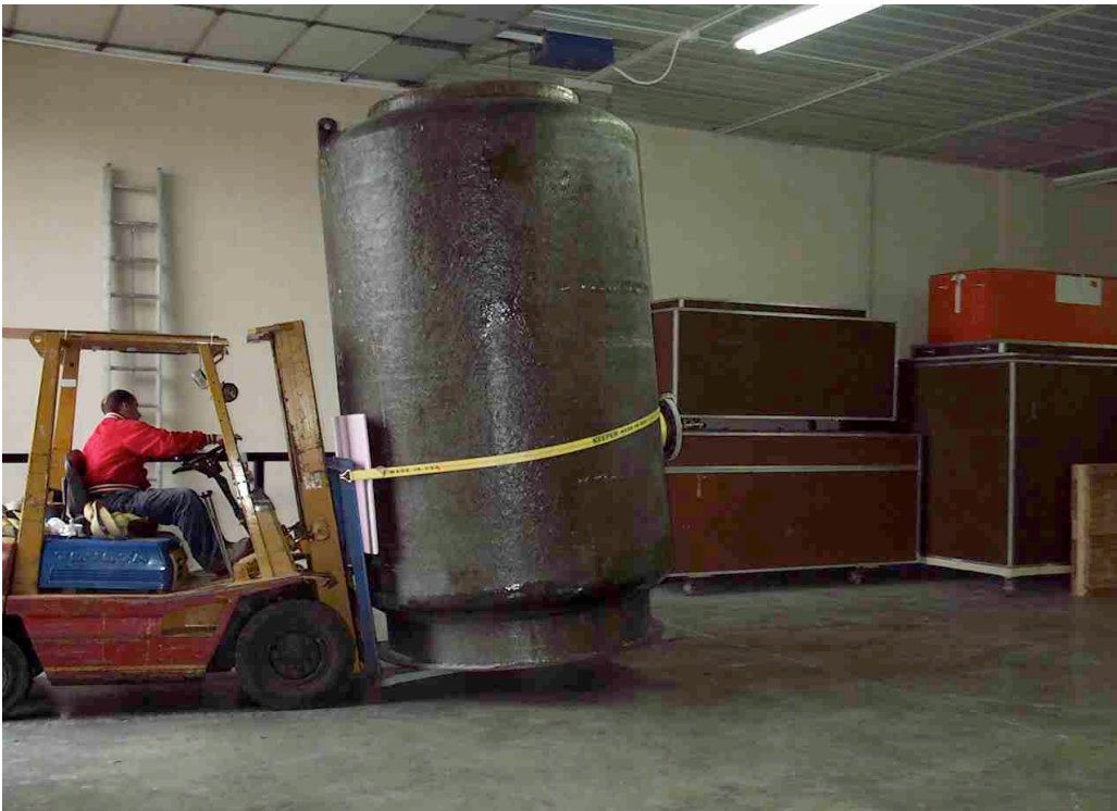
One in a vertical position, the cryostats can be placed on a forklift (pink insulation board used for padding) and returned to the warehouse for positioning.
