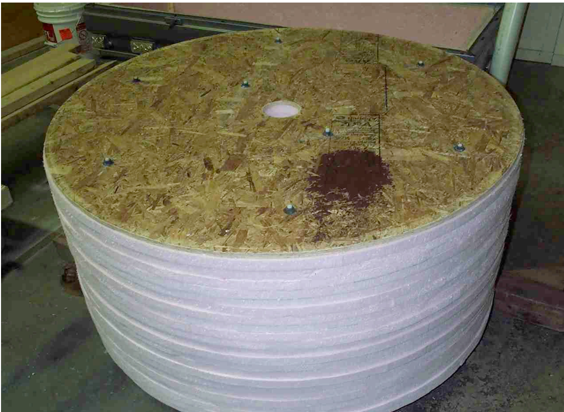
A plastic cylinder is inserted into a hole made in the middle of the pink insulation boards. Plastic rods through the insulation boards and plywood secure the insulation boards.
