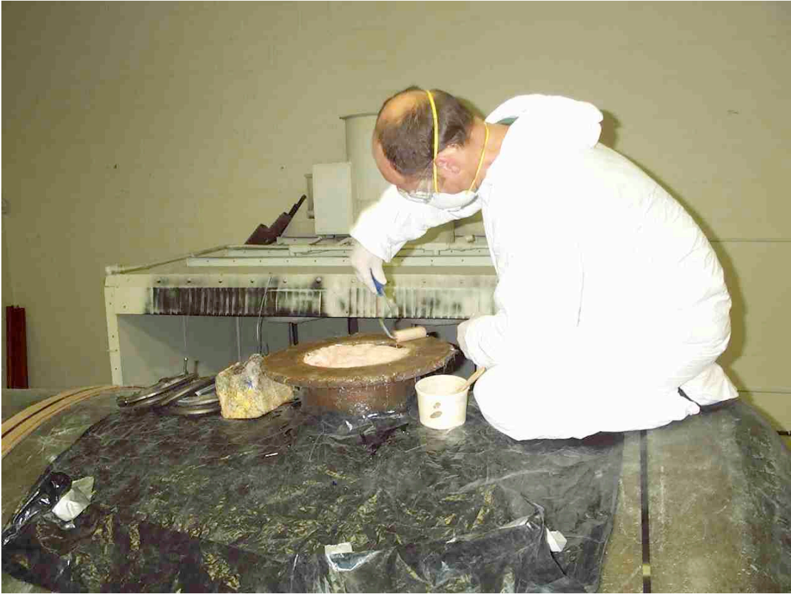
A roller is used to apply more laminating resin to the fiberglass “cloth” rings. Three fiberglass “cloth” rings are applied in this manner to each cryostat. The roller is cleaned with acetone. The filter plate is painted with laminating resin for adherence.
