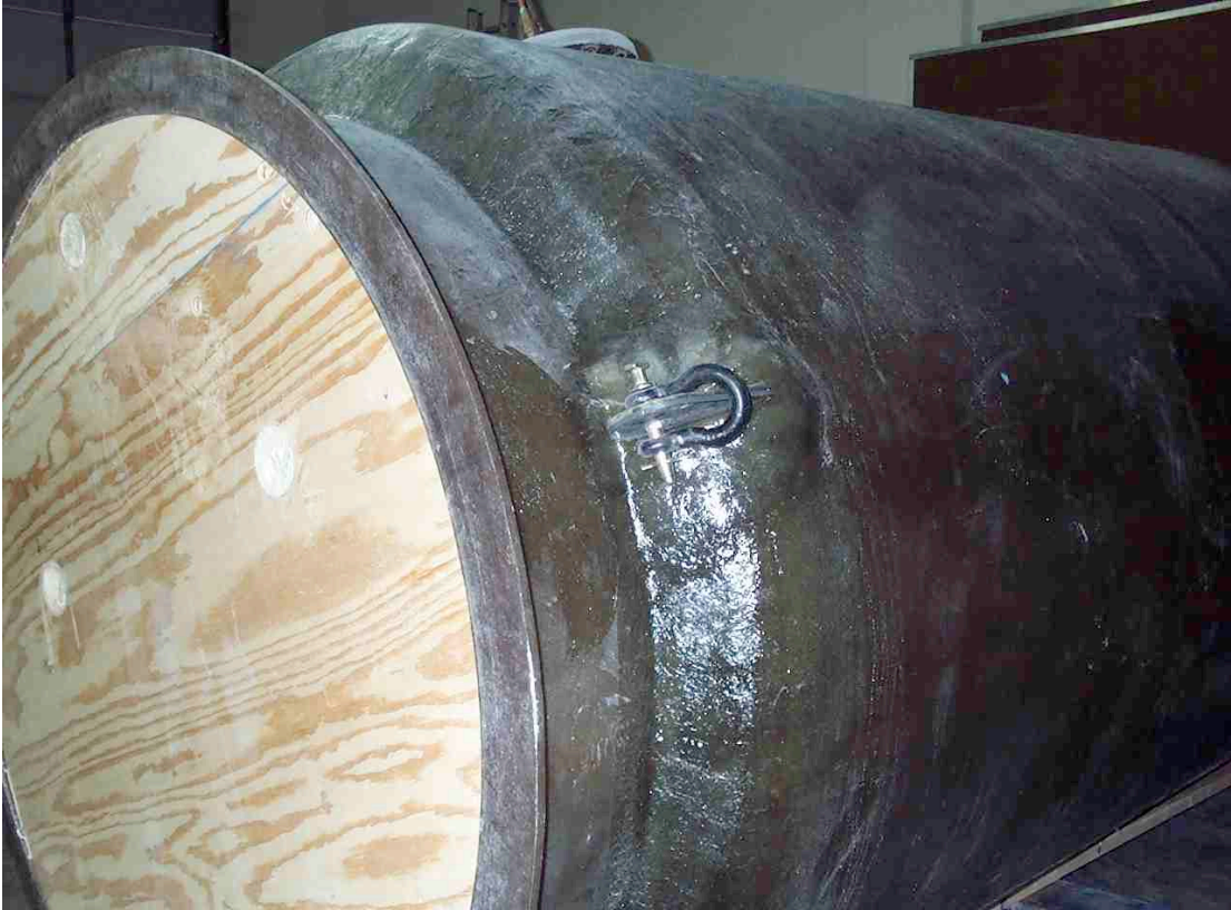
The cryostats are blocked on 4-by-4s to position them for hoisting.
