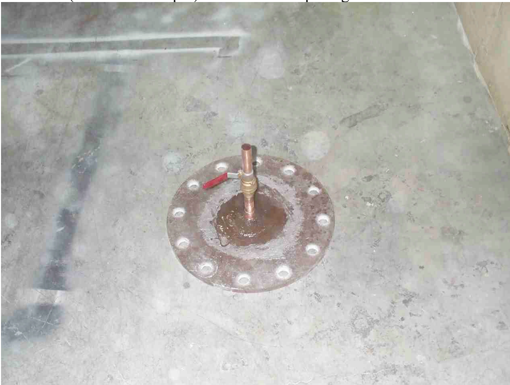
An air hose is used to clean the perlite dust off of the cryostats. The 16½" diameter fiberglass plate for the filter hole is drilled in the center and 11" copper pipe with hand ball valve (from Home Depot) is fitted to the opening.
