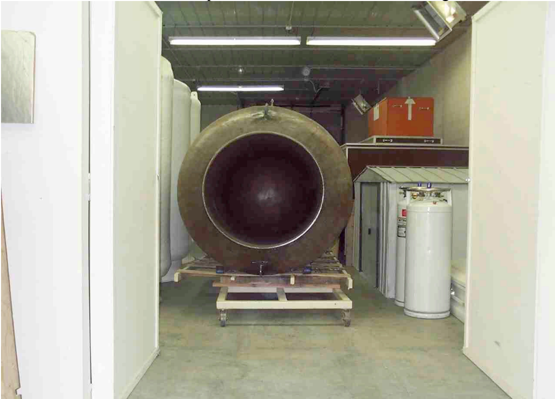
As before the wooden skids are placed on the metal frames for rolling.
