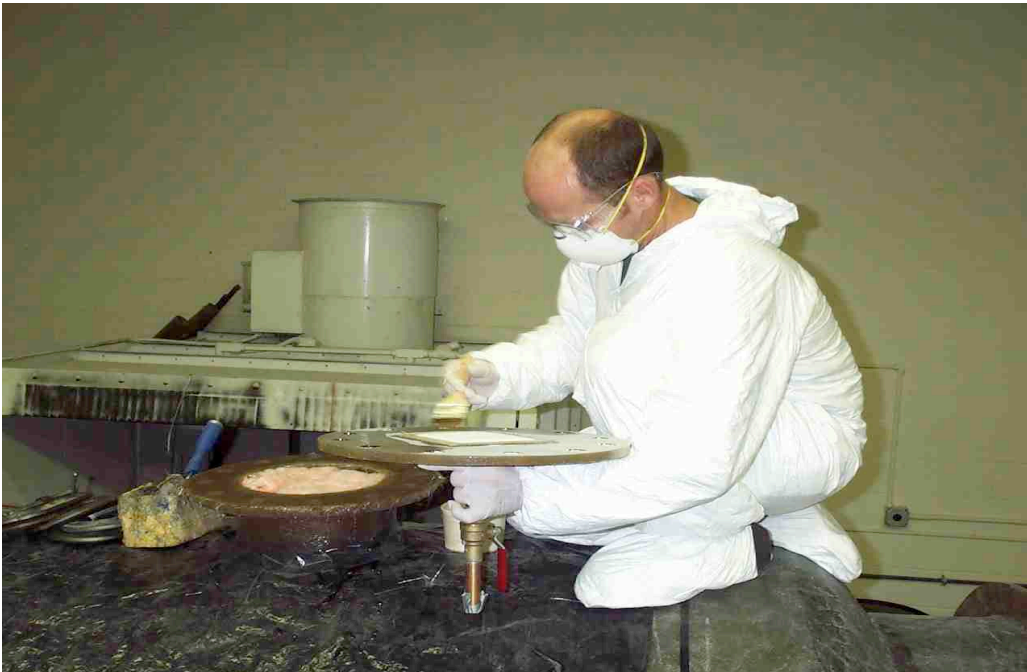
A roller is used to apply more laminating resin to the fiberglass “cloth” rings. Three fiberglass “cloth” rings are applied in this manner to each cryostat. The roller is cleaned with acetone. The filter plate is painted with laminating resin for adherence.
