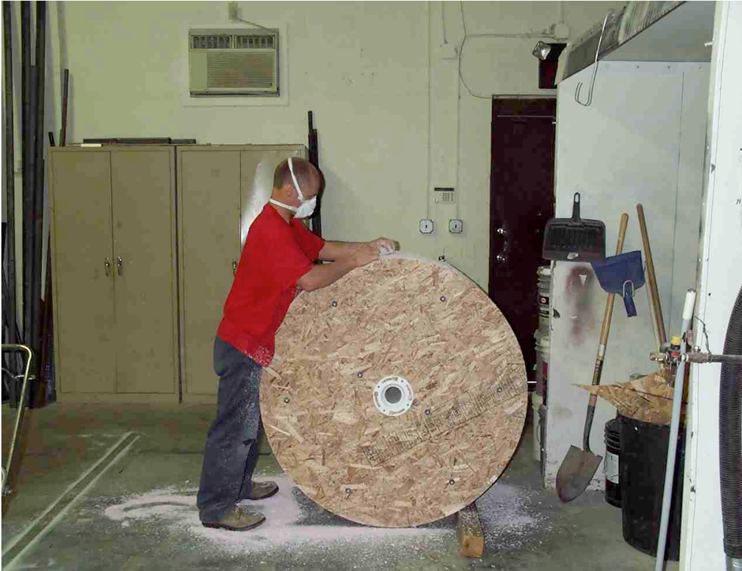
The rim of the insulation boards is scraped/sanded (?) to a fine finish.
