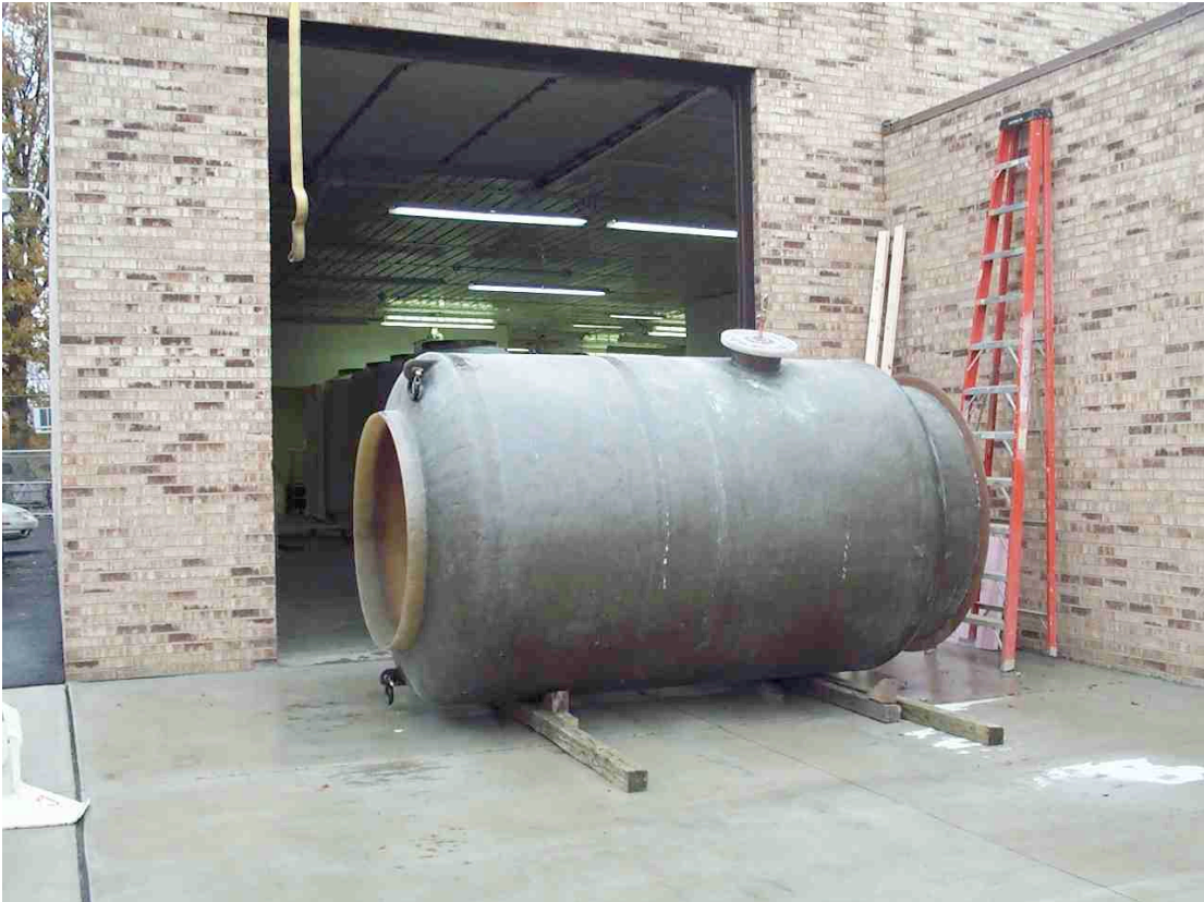
The cryostats are blocked on 4-by-4s to position them for hoisting.
