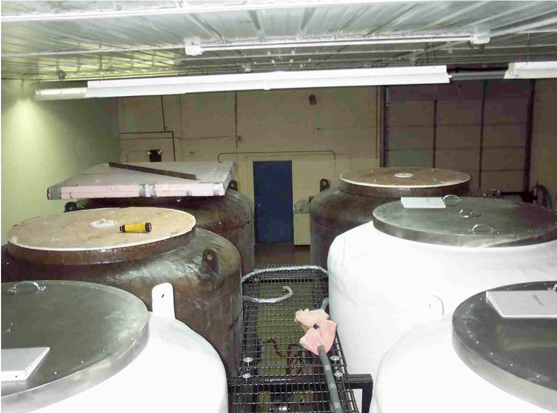
The permanent tops are made from layers of pink fiberglass board that is sandwiched between plywood boards.
