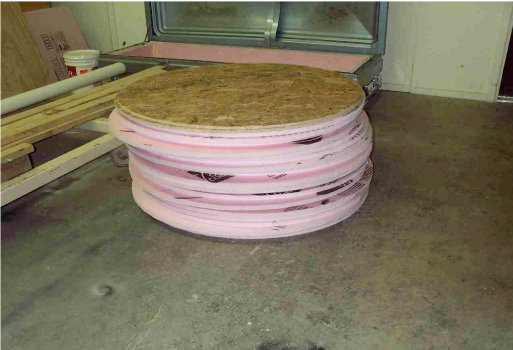
The permanent tops are made from layers of pink fiberglass board that is sandwiched between plywood boards.
