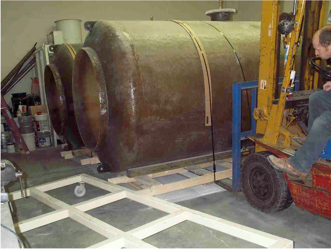
As before the wooden skids are placed on the metal frames for rolling.
